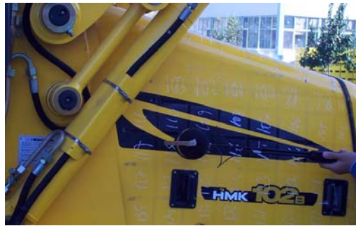
Figure 2 Engine Hood Right Plate Intensity Measurement
