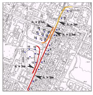
The model was used to define the geometry of the barrier, and to evaluate its efficiency, too. To make that, the model was used to calculate the new noise levels, after both interventions, in the same points of the first measurement campaign. So it was possible to make a comparison between the two situations: the first, related to the "ante-operam" scenario, and the second, to the "post-operam" one.
