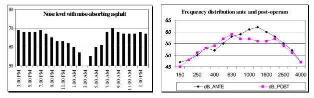
The project of the absorbing/insulating barrier was carried on with the help of the model: after the first calibration step and the simulation of the actual situation, it was used to calculate the contribute of noise-absorbing asphalt to sound abatement to receptors. After that second calibration, the model was used to reproduce the real situation in standard traffic conditions.
