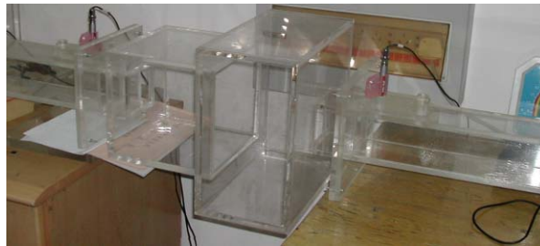
Figure 3. Experimental duct system and the muffler.
