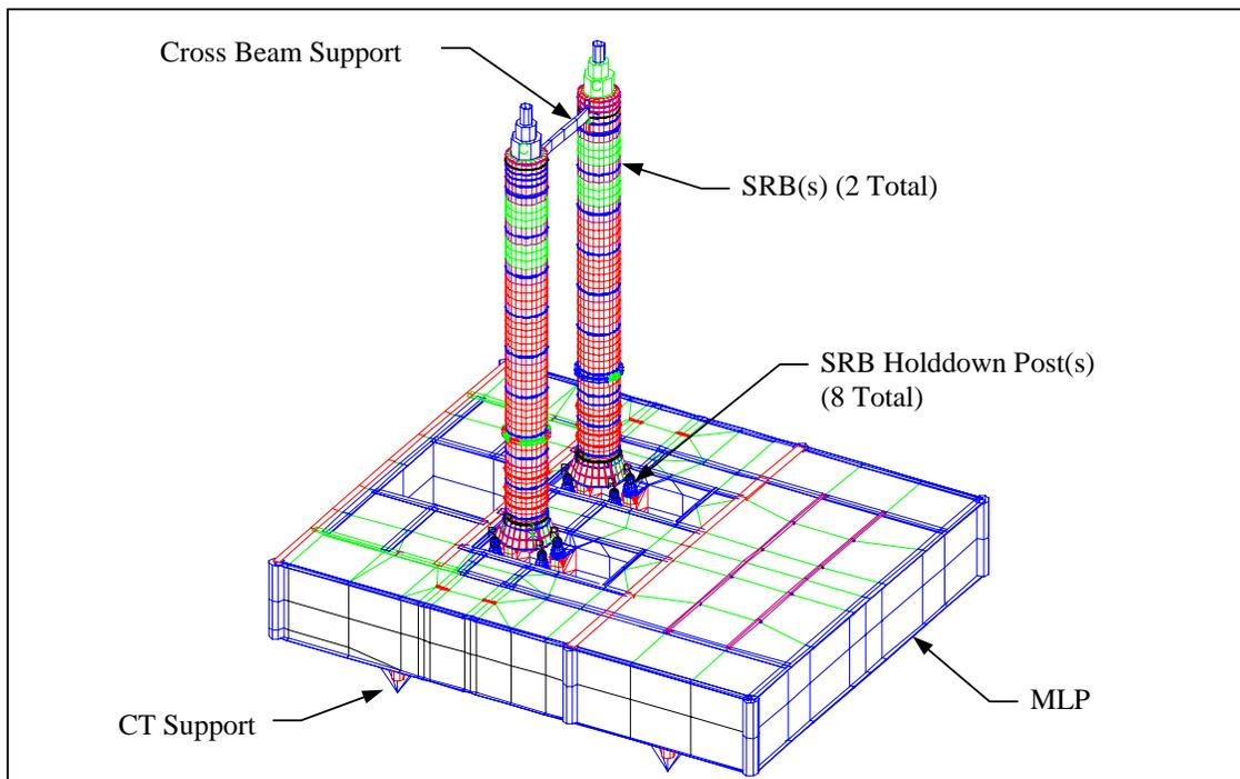
Figure 2. SRB, MLP, and CT Structural Math Model [Reference 1]
