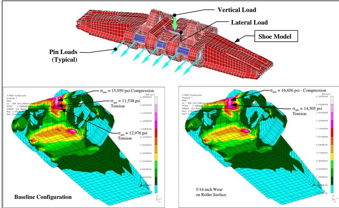
Figure 3. Typical Shoe FE Model used for Stress and Vibration Analysis [Reference 2]
