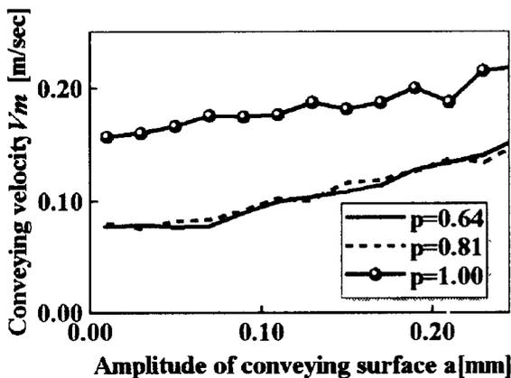
Fig. 6 Effect of flat ratio  $p$
