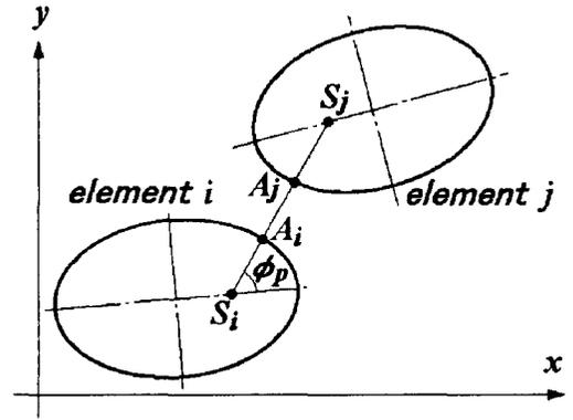
Fig. 3 Distance between two ellipse elements
