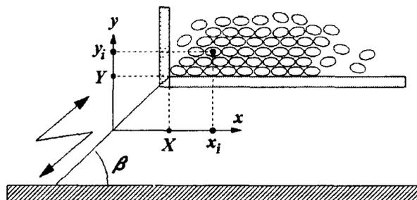
Fig. 1 Model of a vibratory conveyor
