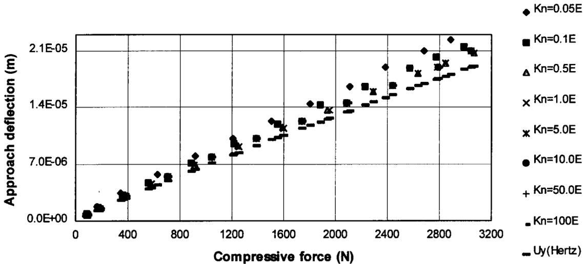
Fig.4 The effect of varying contact stiffness Kn
