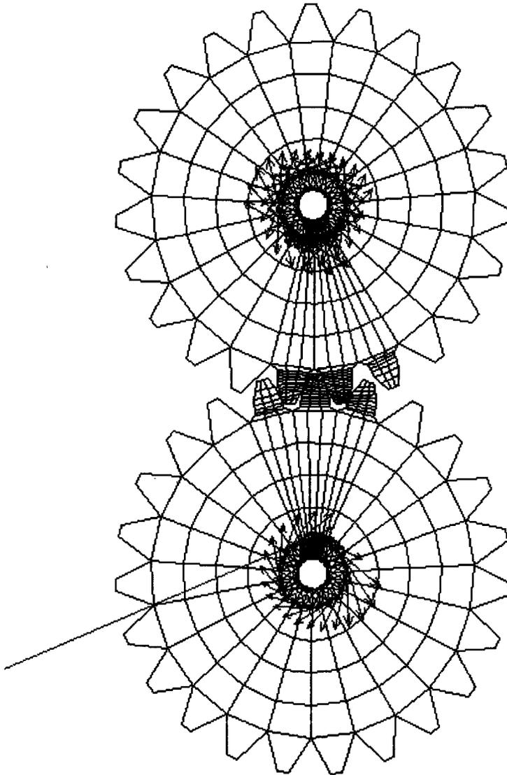
Figure 1. Finite Element Model of the spur gears in mesh with the load and boundary conditions.
