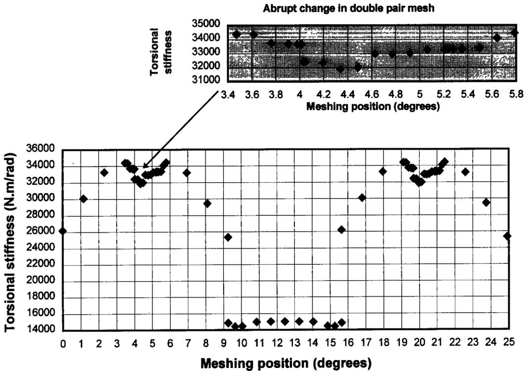
Figure 6. Torsional stiffness (N.m/rad) of one complete mesh cycle
