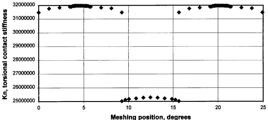
Figure 5. The variation of torsional contact stiffness, Kn over the mesh cycle.
