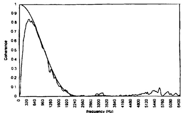
Figure 6: Comparison of measured and computed coherence function for two parallel velocity components 0.10 m apart (from [10]).
