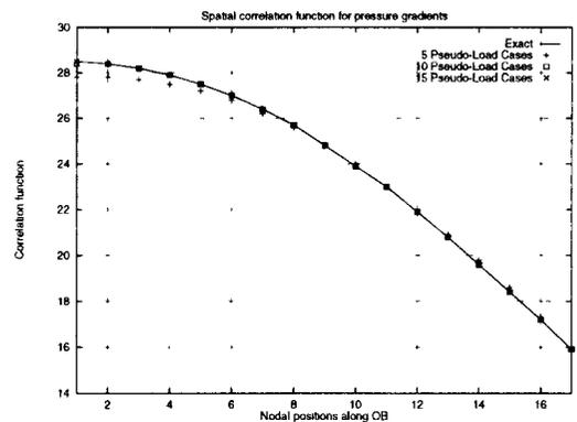
Figure 3(b): Comparison of exact and approximate correlation functions along side OB (at 500 Hz) using 5,10 and 15 pseudo-load cases.
