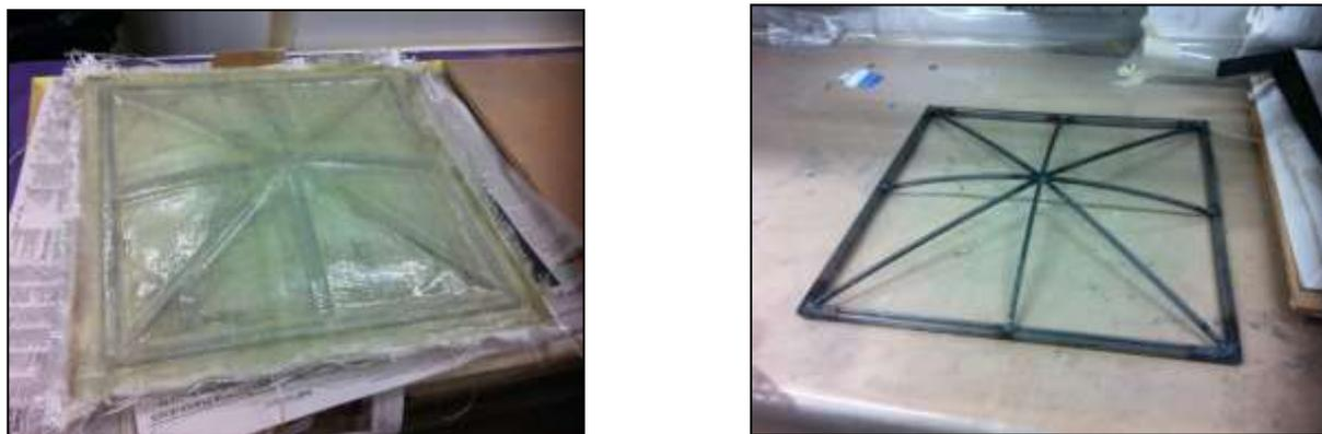
**Figure 7 - welded steel reinforced frame**
