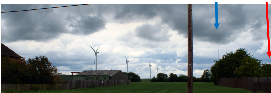
Figure 3 – Post-wind farm showing anemometer (arrowed blue) & microphone location (red) in rear garden of dwelling.
