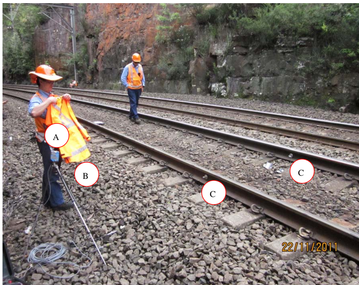
Figure 1 – Measurement system to identify which wheel is squealing – microphone (A), optical switch used as a wheel sensor (B) and rail mounted accelerometers (C)
