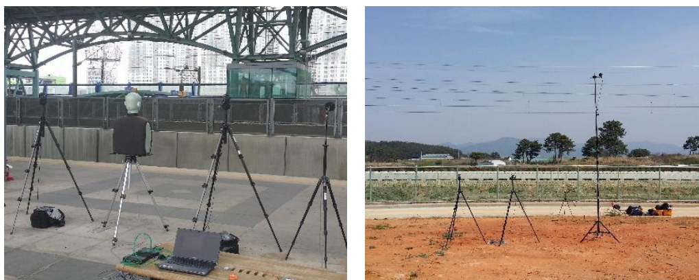
Figure 3 – Noise measurement (left: train station, right: track side)
