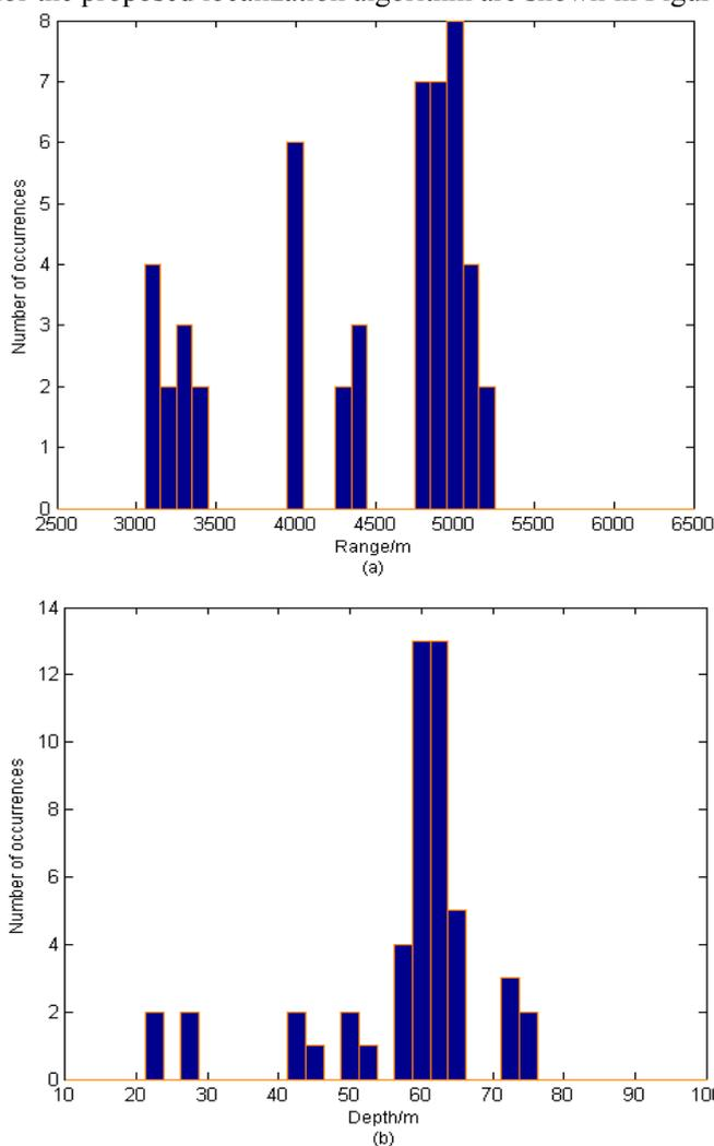
Figure4 Histogram of localization for environmental uncertainty (a) Depth estimation (b) Range estimation
