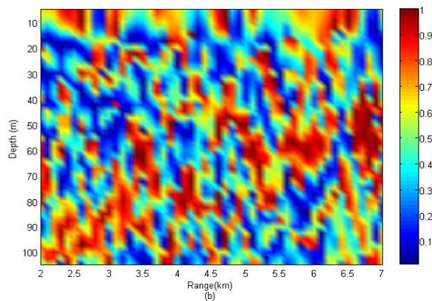
Figure3—Ambiguity surface for (a) CCMFP (b) Bartlett MFP
