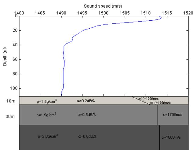
Figure1—Simulated ocean environment model
