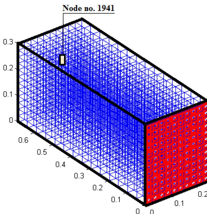
Figure 2 – Finite element mesh of the acoustic domain of the cavity
