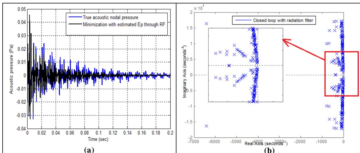
Figure 9 – a) Comparison of open loop and closed loop acoustic pressure b) pole-zero map
