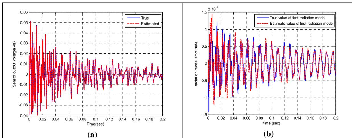
Figure 8 – Comparison of true and estimated a) piezoelectric sensor voltage b) modal amplitude of first radiation mode
