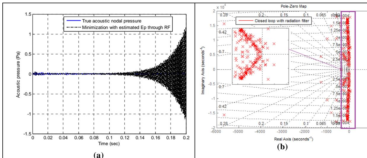
Figure 6 – a) Comparison of open loop and closed loop acoustic pressure b) pole-zero map
