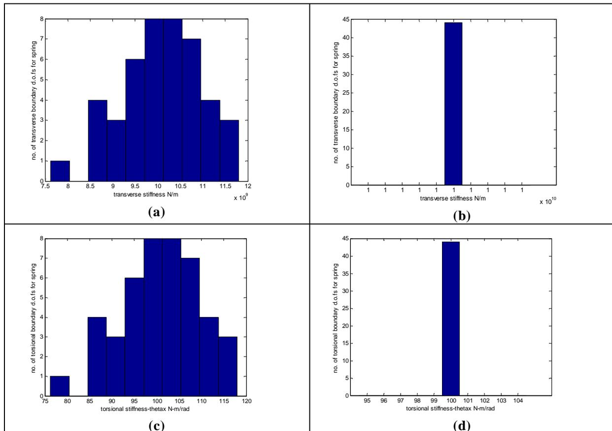
Figure 7 – Stiffness distribution at the boundary of the plate a) Transverse stiffness in plant model b) Transverse stiffness in Kalman filter model c) torsional stiffness in Plant model d) torsional stiffness in Kalman filter model
