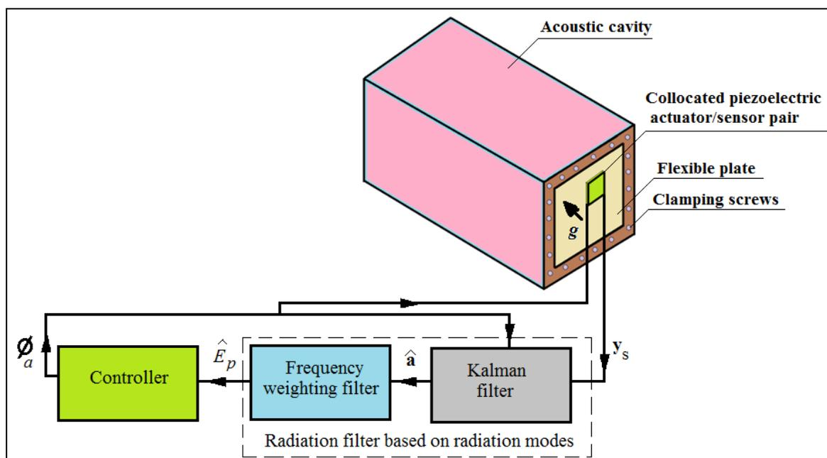
Figure 1 – Schematic representation of feedback control of interior sound
