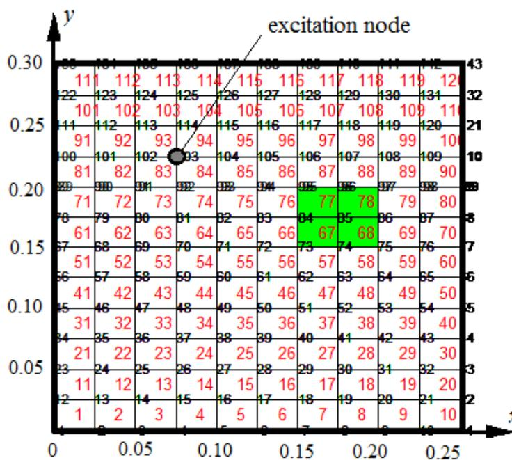
Figure 3 – Finite element mesh of the structure with piezoelectric patches
