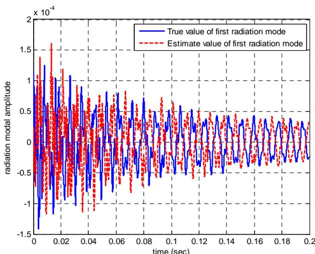
Figure 5 – Comparison of true and estimated value of modal amplitude of first radiation mode
