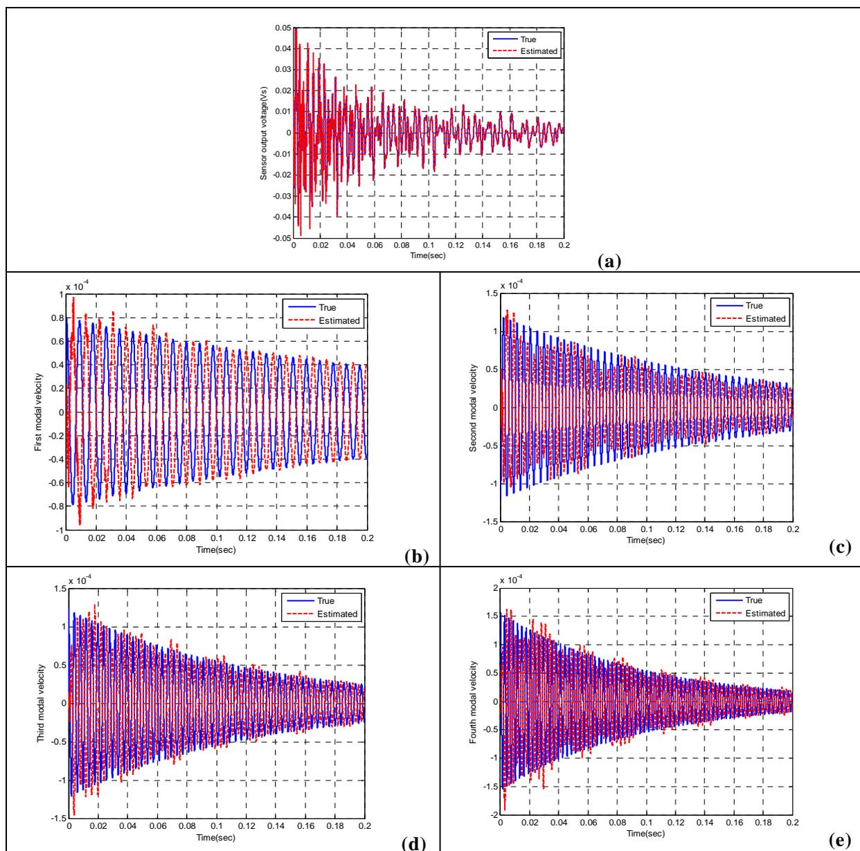
Figure 4 – Comparison of true and estimated values of a) piezoelectric sensor voltage and b)-e) modal velocity of structural modes
