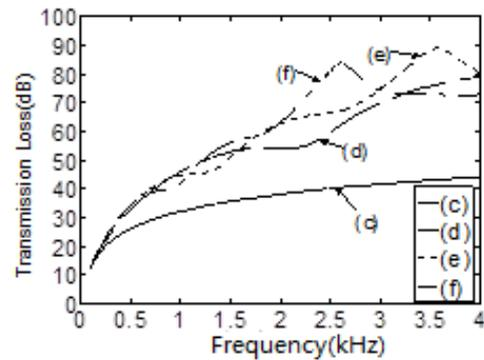
Figure 4 –TL of different thickness of porous material
