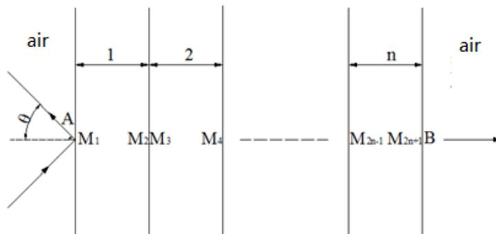
Figure 2 – Plane wave incidence of multi-layer composite medium
