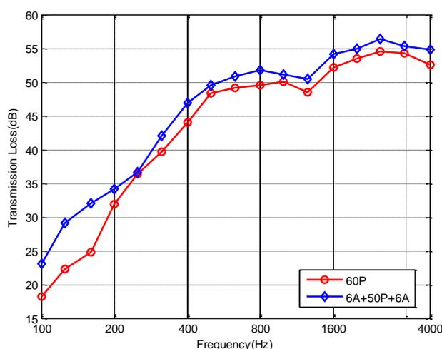
Figure 7. Transmission loss curves of experimental testing in reverberation room for different materials
