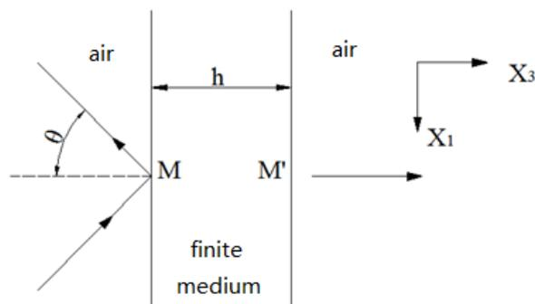
Figure 1 – Plane wave incidence of single layer medium with  $h$  thickness
