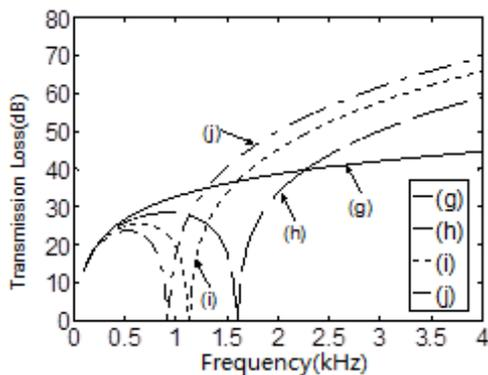
Figure 5 –TL of different thickness of air layer
