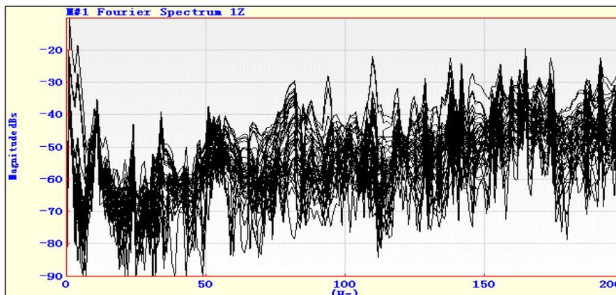
Figure 6 – Transfer function of acceleration/force of floor skeleton below 200Hz
