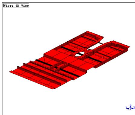
(b) Surface model of the bottom floor
