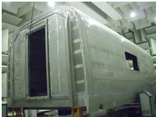
Figure 1 – 7 meters carriage BIW
