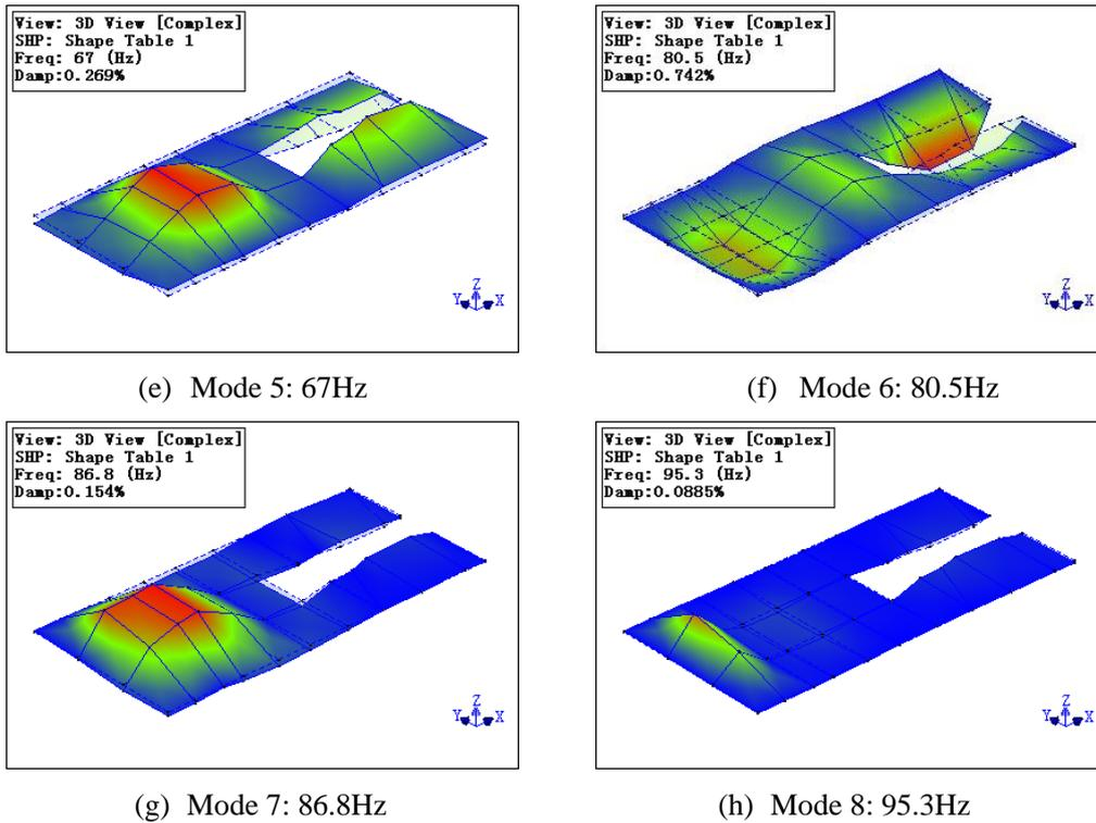
Figure 8 – Mode shapes of floor skeleton
