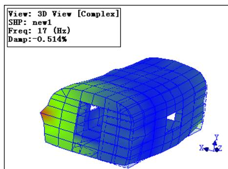
(b) Bending mode shape perpendicular to Y axis
