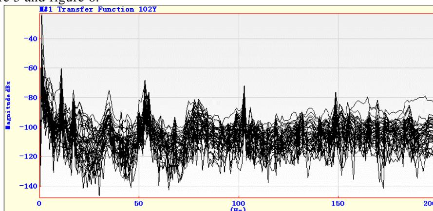
Figure 5 – Transfer function of acceleration/force of the carriage model below 200Hz
