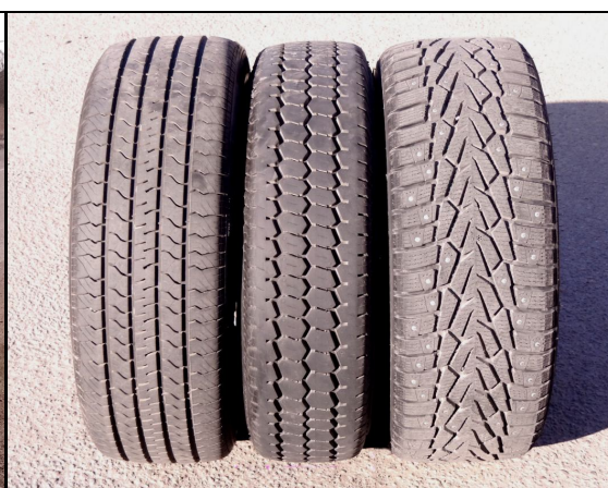
Figure 5. The three test tyres used during the CPX noise tests. From left to right: SRTT, AV4, H7WS. The latter winter tyre was used only in the late-winter tests. Its steel studs can be weakly seen as bright spots near the shoulders.
