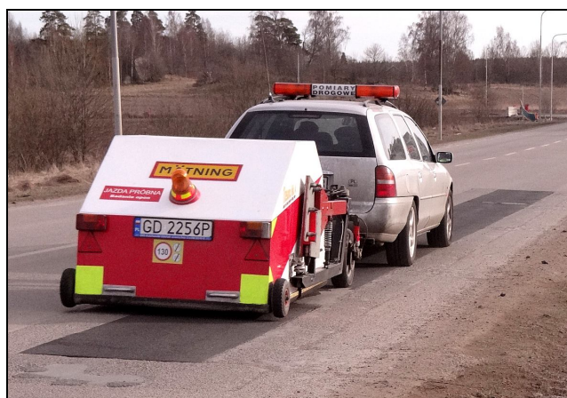
Figure 4. CPX noise tests with the TUG Tiresonic Mk.4 trailer on the 25 m long PERS section in Linköping in March 2014. The test tyre is mounted in the middle of the chamber.
