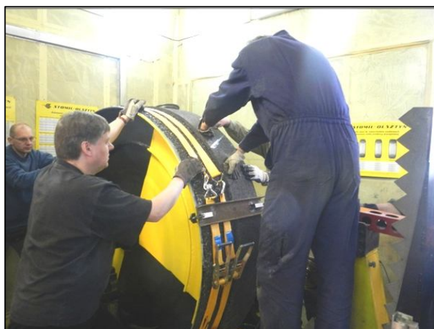
Figure 1. Mounting of the PERS sheets on the test drum for car tyres.
