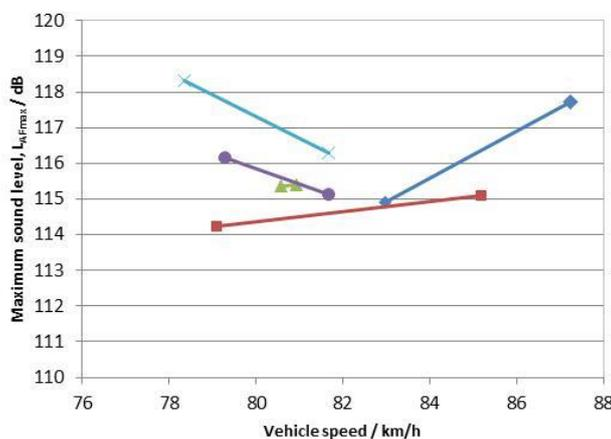
Figure 6 – Changes in  $L_{AFmax}$  with test vehicle speed
