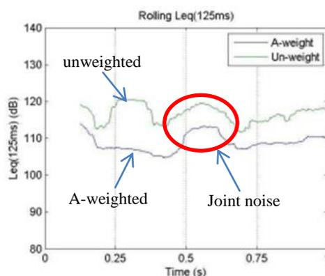
Figure 4 – Comparison of A-weighted and unweighted noise data
