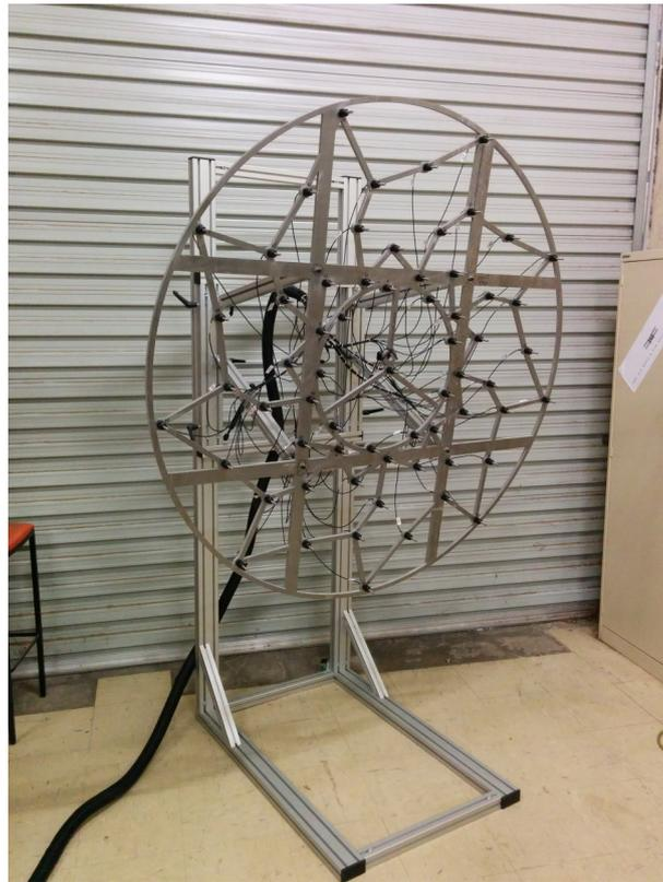
Figure 4 – The assembled School of Mechanical Engineering beamforming array.
