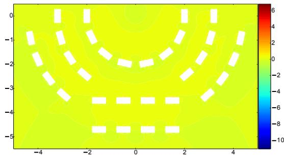
Figure 9 –  $\Delta L$  for 62.5 Hz (1/3 octave band) for standard orchestra configuration.
