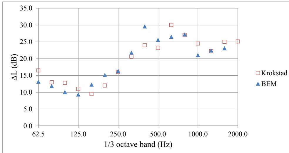
Figure 6 – Comparison of  $\Delta L$  (average  $\Delta L$  for source heights 0.6 m, 0.9 m and 1.3 m) varying with 1/3 octave bands from full scale measurements and BEM model.
