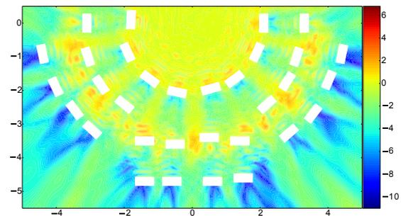
Figure 16 –  $\Delta L$  for 1000 Hz (1/3 octave band) for orchestra configuration with random perturbations introduced.
