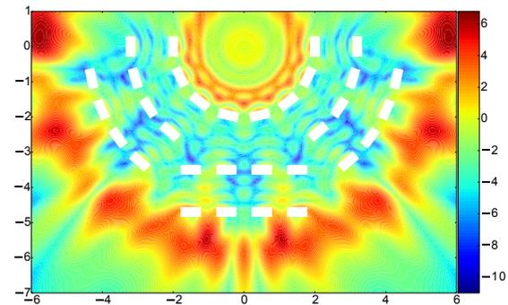
Figure 12 –  $\Delta L$  for 500 Hz (1/3 octave band) for standard orchestra configuration.
