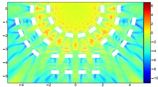
Figure 13 –  $\Delta L$  for 794 Hz (1/3 octave band) for standard orchestra configuration.
