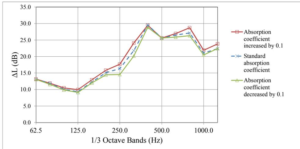
Figure 5 – Effect of increasing and decreasing absorption coefficient by 0.1 on  $\Delta L$  for the setup of Figure 1.
