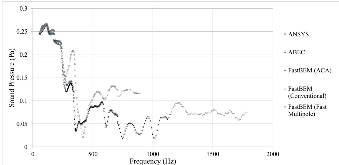
Figure 3 – Comparison of sound pressure at 8 m from source for configuration used by Krokstad. Results are from ANSYS, ABEC and FastBEM (3 different solvers). Note the discontinuities relate to changes in complex impedance.
