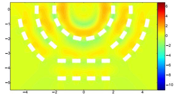
Figure 10 –  $\Delta L$  for 125 Hz (1/3 octave band) for standard orchestra configuration.
