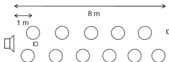
Figure 1 – A plan view of configuration used by Krokstad, with larger circles represented musicians heads and smaller circles representing microphone locations - image taken from (7).
