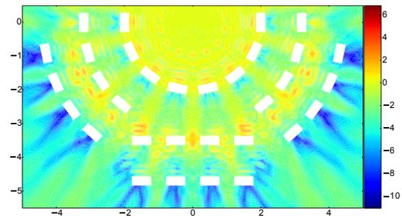
Figure 14 –  $\Delta L$  for 1000 Hz (1/3 octave band) for standard orchestra configuration.
