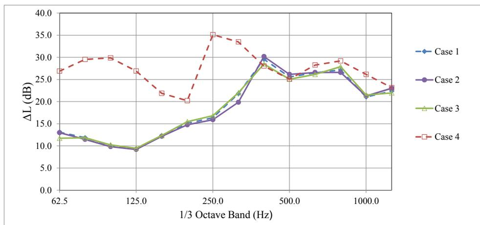
Figure 4 – Effect of altering real and imaginary complex impedance components on  $\Delta L$  for the setup of Figure 1. See Table 1 for definitions of Cases 1–4.
