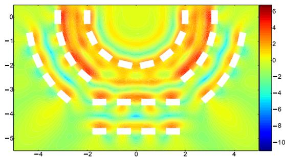
Figure 11 –  $\Delta L$  for 250 Hz (1/3 octave band) for standard orchestra configuration.
