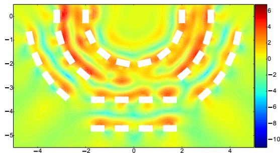
Figure 15 –  $\Delta L$  for 250 Hz (1/3 octave band) for orchestra configuration with random perturbations introduced.
