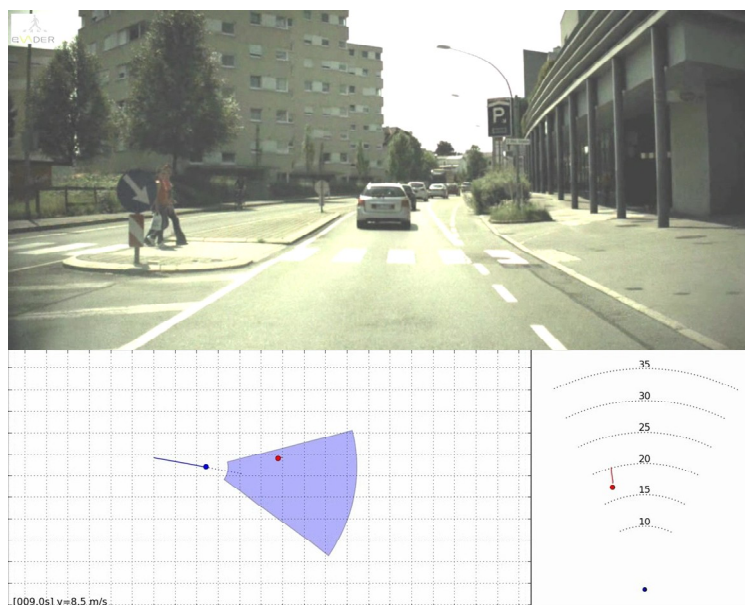
Figure 2: eVADER EPS camera view & pedestrian detection simulation result (Source eVADER consortium members AIT and Continental)
