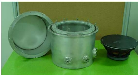
Figure 3 - Cavity and loudspeaker constitutive parts of the infrasound calibrator.
