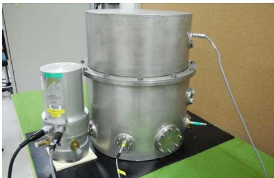
Figure 4 - The infrasound calibrator in the comparison method configuration.
