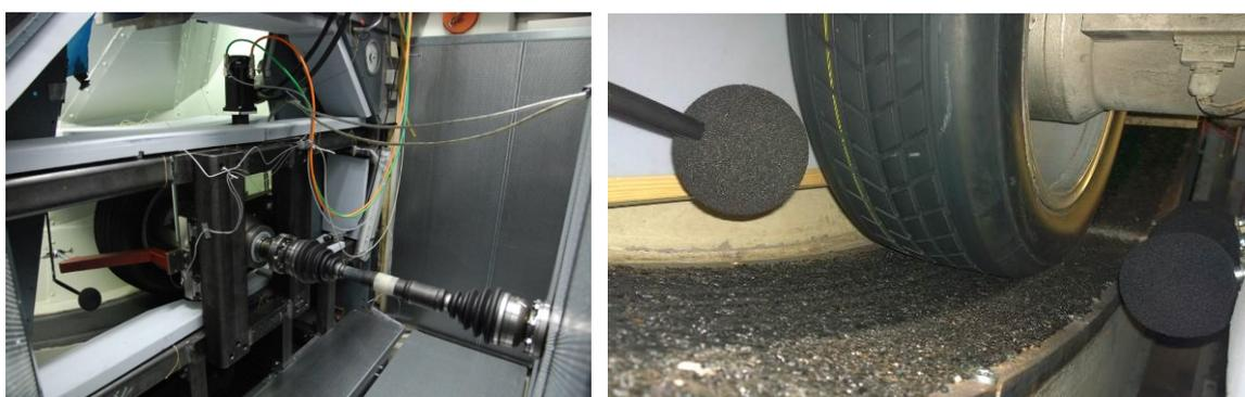
Figure 2 - Acoustically optimised inner drum test facility using real road pavement at KIT
