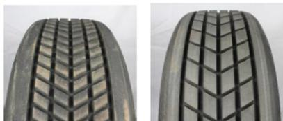
Figure 5 - Different geometry of tread pattern (R11 left, R12 right).
