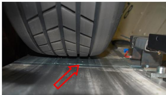
Figure 3 - Triaxial force sensor placed in a road surface in the internal drum test facility.
