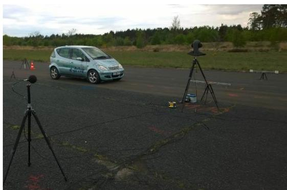
Figure 4 - The KIT electric vehicle passing the measuring setup at Geilenkirchen, Germany.
