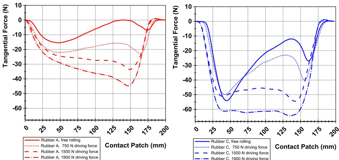
Figure 8 - Comparison of force curves of different rubber compounds under driving torque conditions, (0 mm = leading edge, Rubber A left, Rubber C right)
