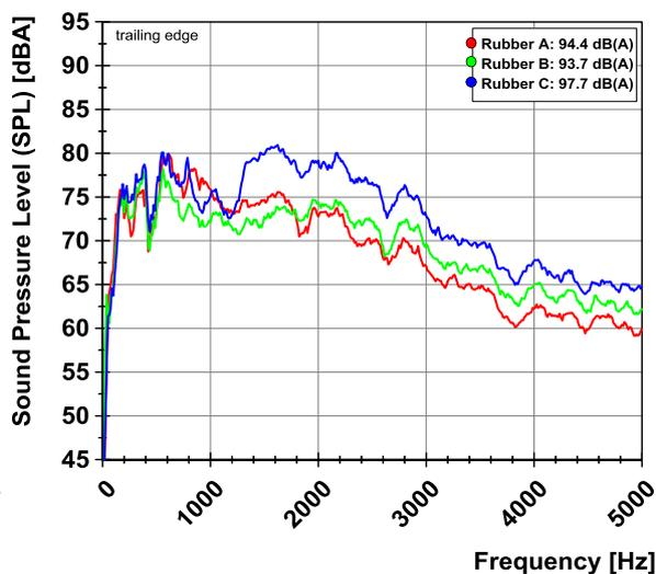
Figure 7 - Comparison of tire compounds, 3500 N circumferential force, 30 km/h, SMA 8, trailing edge.
