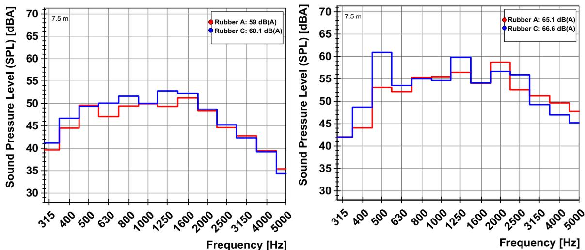
Figure 9 - Sound level generated during coast-by (left) and during accelerated pass-by (right) for different tire tread compounds.
