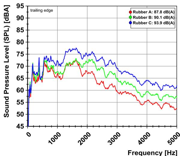
Figure 6 - Comparison of tire compounds, coasting, 30 km/h, SMA 8, trailing edge.
