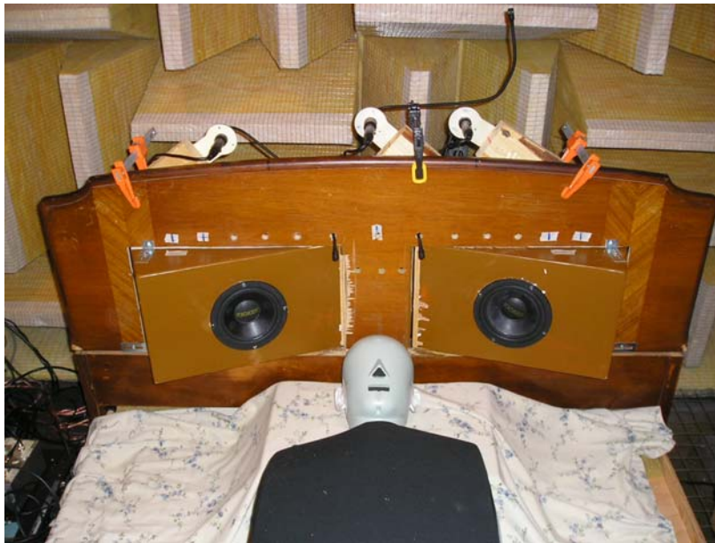
Fig. 2. Experimental setup of the snore ANC system based on the headboard.
