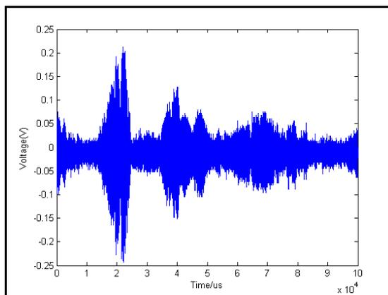
Fig.4 The Doppler signal after mixing
