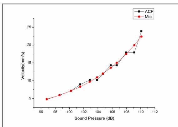
Fig.9 ACF with 50 kHz mixing
