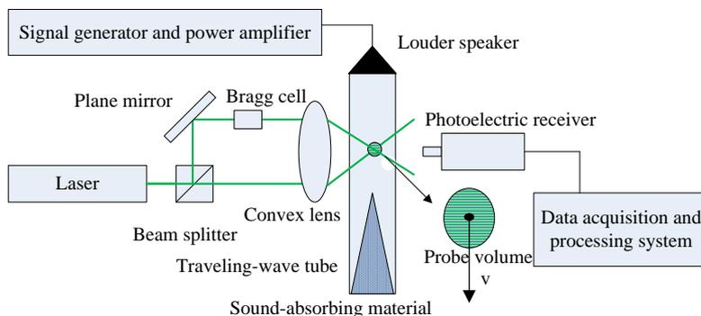
Fig.1. Schematic diagram of LDA
