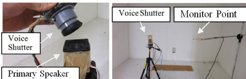
Figure 7– Experimental set up for speaker voices
