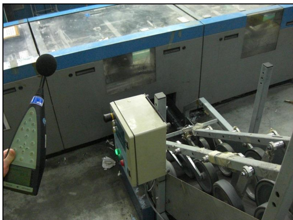
Figure 11. Press waste chute (rattling panel below at ground level beneath control box)
