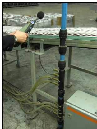
Figure 8. Leaky air line
