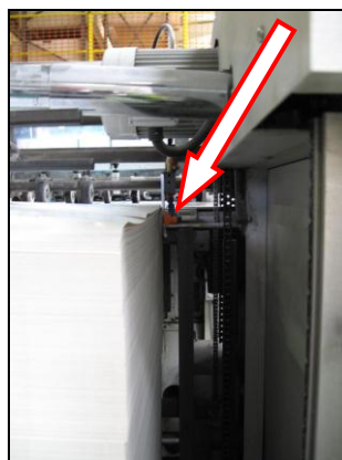
Figure 9. Leaky air nozzle
