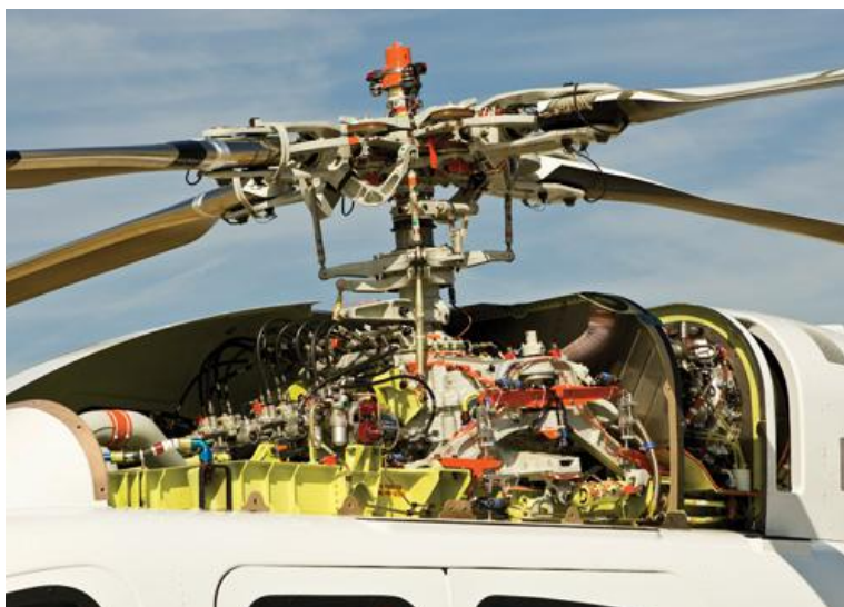
Figure 1 – View of the inside of the transmission region in a commercial rotorcraft.
