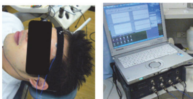
Figure 1–Measurement system with headband type microphones.
