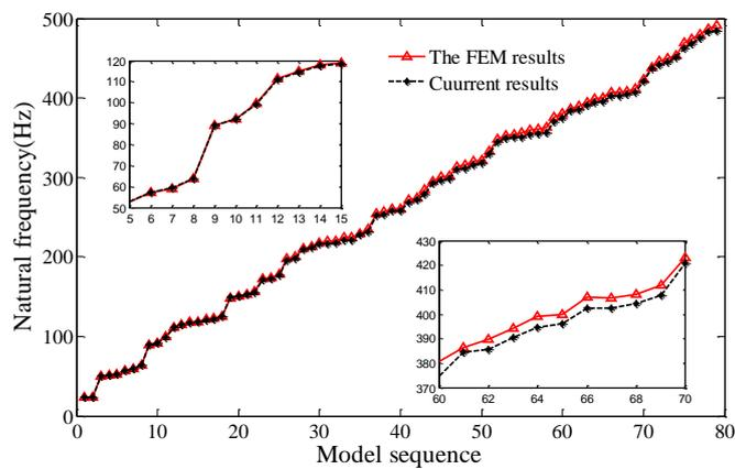
Figure 6 – Comparison of natural frequencies between the present method and the FEM with the boundary condition (d)
