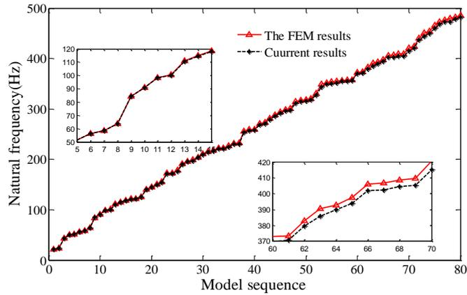
Figure 5 – Comparison of natural frequencies between the present method and the FEM with the boundary condition (c)
