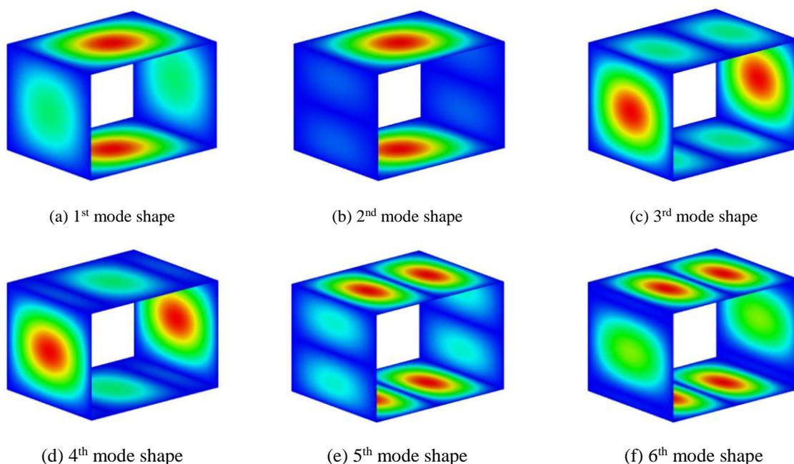
Figure 8 – The first six mode shapes calculated by ABAQUS with the boundary condition (b)
