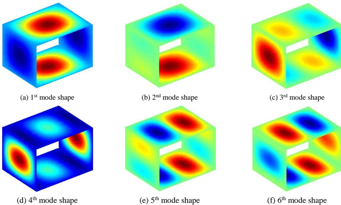
Figure 7 – The first six mode shapes calculated by present approach with the boundary condition (b)
