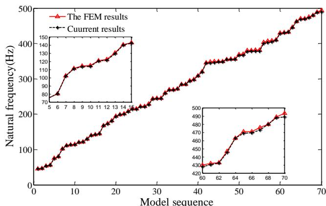
Figure 4 – Comparison of natural frequencies between the present method and the FEM with the boundary condition (b)
