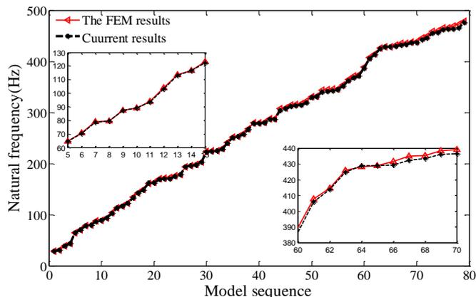
Figure 3 –Comparison of natural frequencies between the present method and the FEM with the boundary condition (a)
