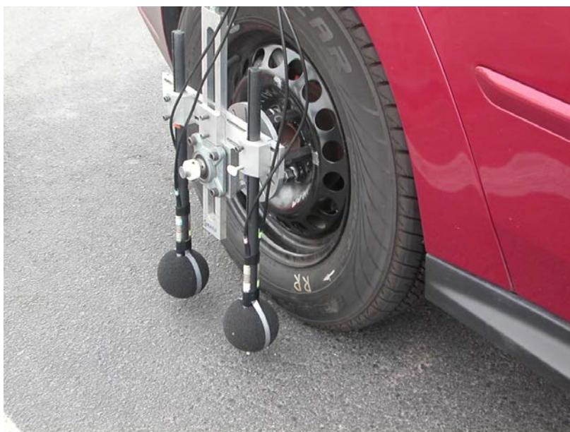
Figure 1 – OBSI test fixture mounted on test vehicle with a Goodyear Aquatred 3 test tire
