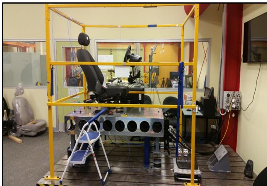
Figure 1 – This Motion-based vibration simulator was developed for the human drowsiness assessment. Actual vehicle seat was mounted on a vibration table. The hydraulic actuator was located off-centre of the table to provide multi-axial input
