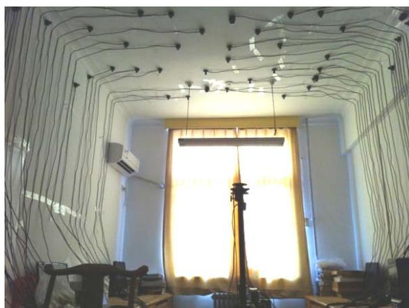
Figure 7 – Setup of randomly distributed microphone array mounted on the ceiling
