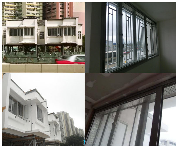
Figure 3 – Mock-up Test of Plenum Type Acoustic Window Design
