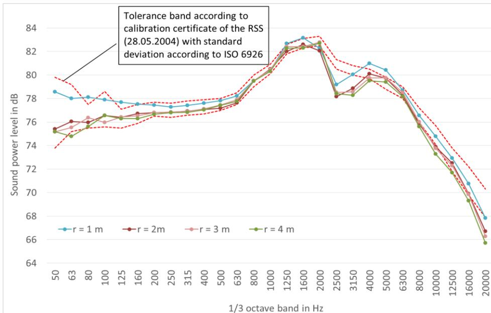
Figure 5 Averaged spectra of sound power level measurements of a B&K reference sound source (RSS) determined from sound pressure level measurements at 20 microphone positions on a hemispherical measurement surface with different radii. The averaged spectra result from 15 measurements each for the 2m and 4m radius, from 8 measurements for the 3m radius and 10 measurements at a radius of 1 m
