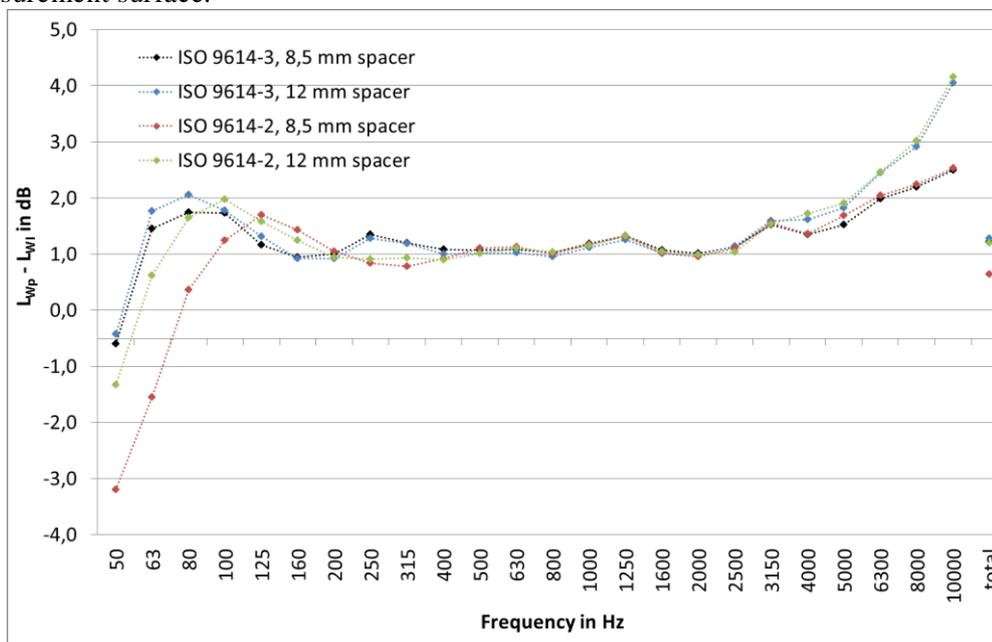
Figure 8 Mean differences of the sound power of the RSS determined from sound pressure respectively sound intensity scanning measurements in 1/3 octave bands according to ISO 9614-2 or -3 using two different spacers.
