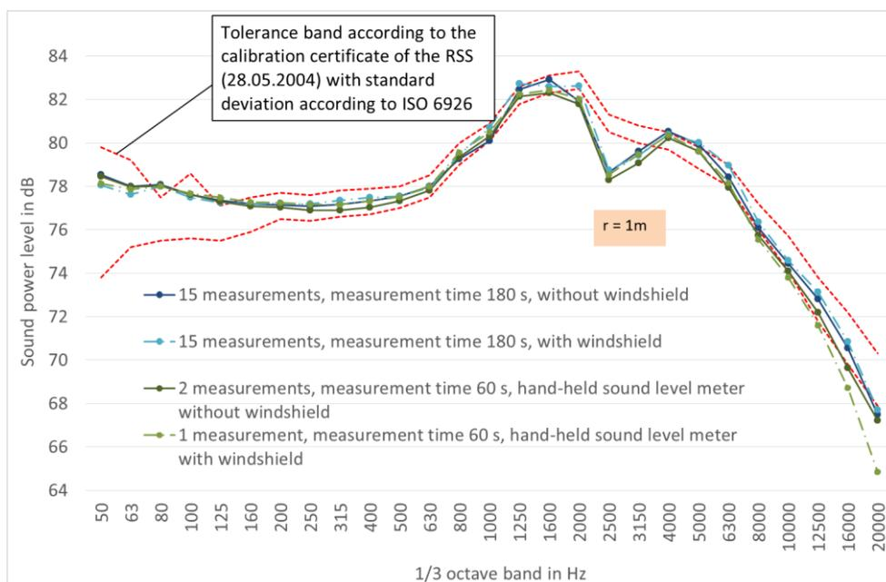
Figure 6 Spectra of the sound power level of a B&K reference sound source (RSS) determined from sound pressure level measurements at 20 microphone positions on a hemispherical measurement surface with a radius of 1m by applying a multi-channel real time measurement equipment or a hand-held sound level meter with pressure level meters of class 1 with windshields attached or not attached to the microphones. The windshield influence was corrected as recommended by B&K.
