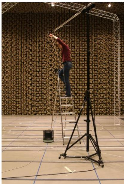
Figure 1 Hemi free-field room used for the sound power level determination
