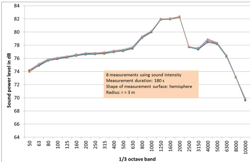
Figure 7 Spectra of 8 sound power level measurements of a B&K 4204 reference sound source (RSS) determined from the normal component of the sound intensity at 20 microphone positions on a hemispherical measurement surface
