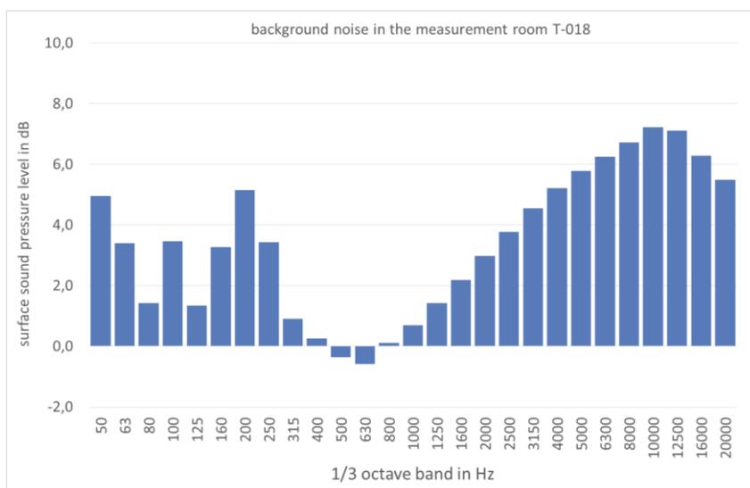
Figure 2 Background noise in terms of the average sound pressure level on the hemispherical respectively on the hemispherical measurement surface in the hemi free-field room determined by using the B&K “Pulse” analyzer
