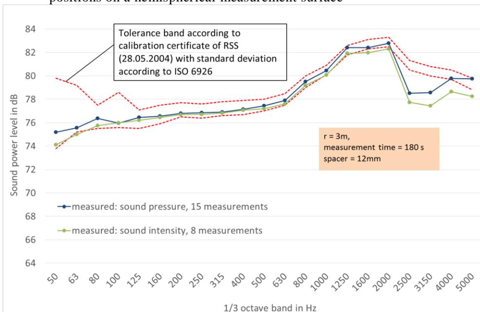
Figure 8 Comparison of the averaged determined sound power level spectra of a B&K reference sound source (RSS) determined from sound pressure and sound intensity measurements at 20 microphone positions on a hemispherical measurement surface with a radius of 3m.
