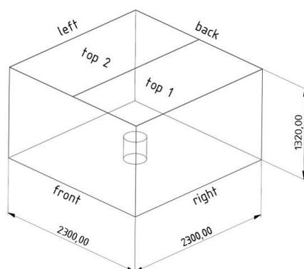
Figure 9 Dimensions of the applied parallelepiped measurement surface including the equal division of the top area
