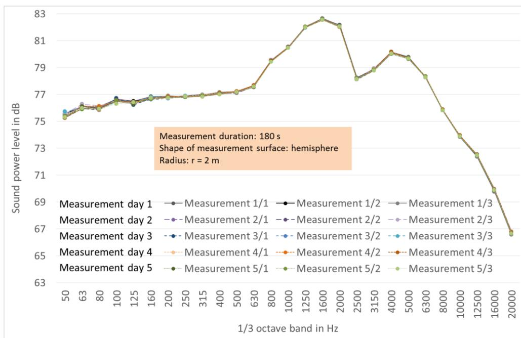
Figure 4 Spectra of in total 15 sound power level measurements of a RSS determined from sound pressure levels at 20 microphone positions on a hemispherical measurement surface
