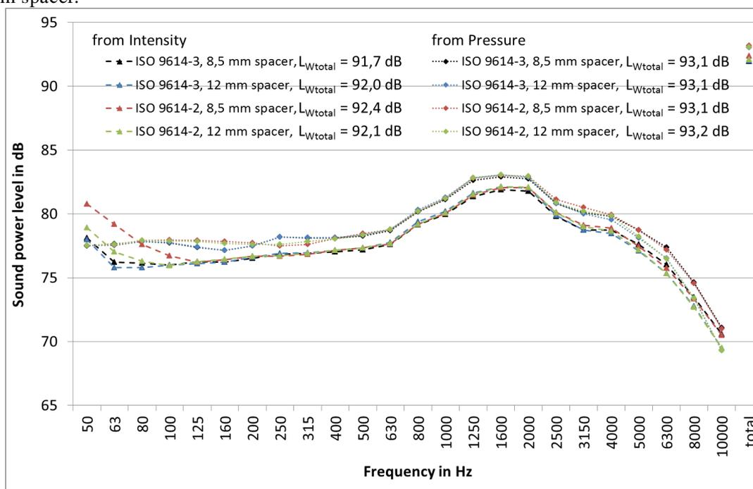
Figure 7 Mean 1/3 octave band sound power level spectra determined from scanning measurements using sound pressure respectively sound intensity, with the latter performed according to ISO 9614-3 respectively ISO 9614-2 applying a 8,5 mm respectively a 12 mm spacer on a parallelepiped measurement surface. The sound pressure used was that directly provided by the analyzer.
