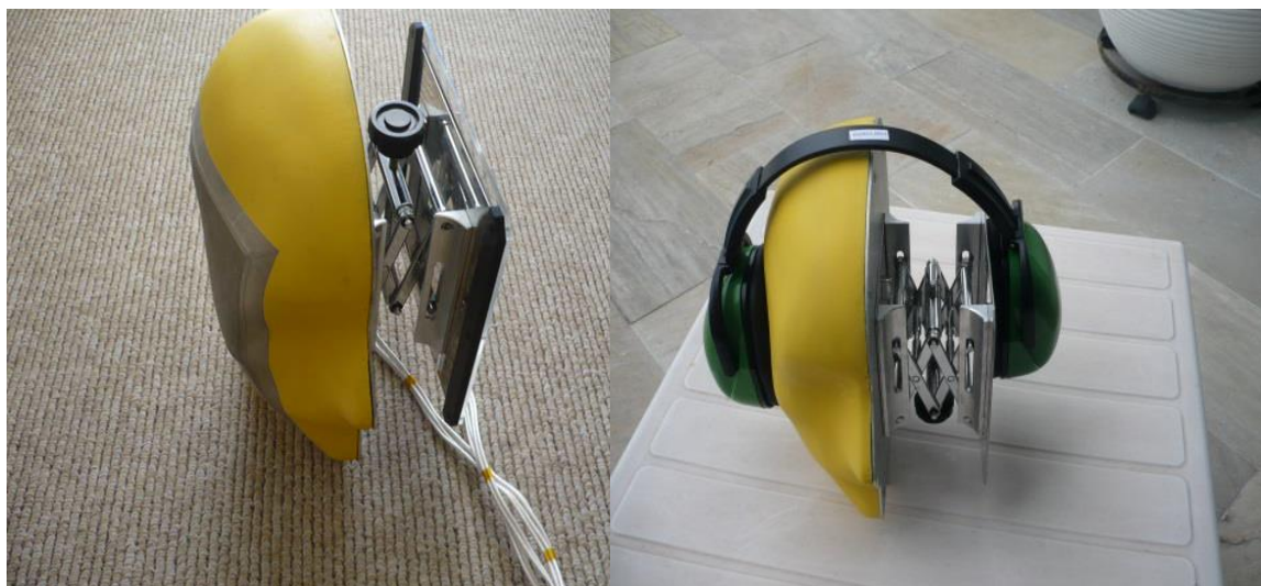
Figure 2 – Variable width measurement systems with flat surface on one side and half human dummy head on the other.
