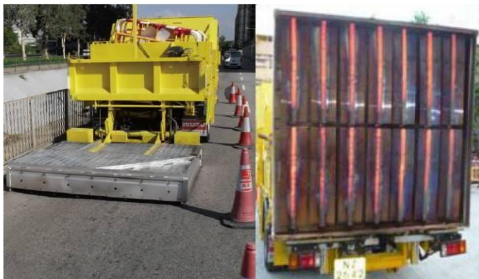
Figure 10 – Removal/Repaving of Asphalt by Infra-red Heating Device
