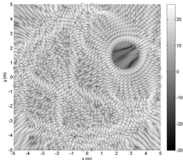
**Figure 6: Reproduction error in dB at 1 kHz,  $R_S = 10$  m,  $R_Z=1$ m,  $\phi_q=30^\circ$ . LWE = 8.7**
