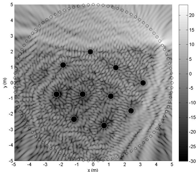
**Figure 7: Reproduction error in dB at 1 kHz,  $f_{Nyq} = 1.3$  kHz, 10 zones,  $R_S = 5.1$  m,  $L = 100$ ,  $LWE=1.2$**
