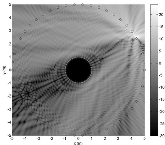
**Figure 4: Reproduction error in dB at 1 kHz,  $R_S = 5.1$  m,  $R_Z=1$ m at origin.  $LWE = 0.76$**
