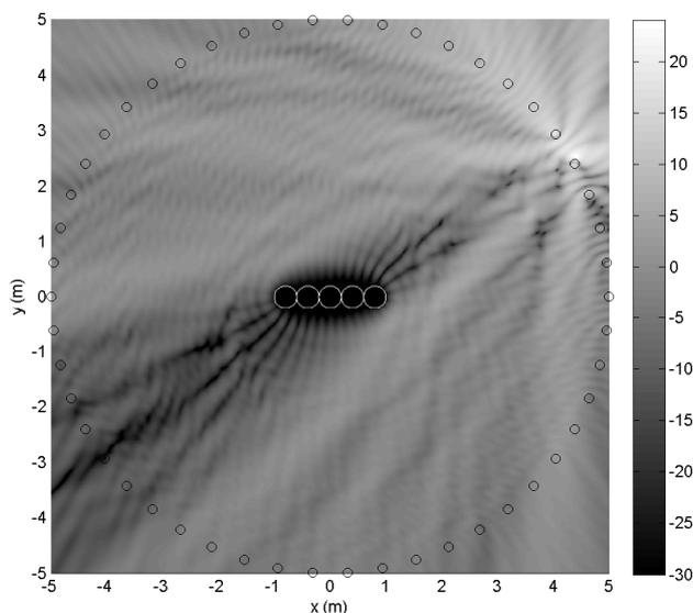
**Figure 8: Reproduction in dB at 1 kHz,  $f_{Nyq} = 1.2$  kHz, 5 adjacent zones,  $R_S = 5.1$  m.  $LWE = 0.53$**
