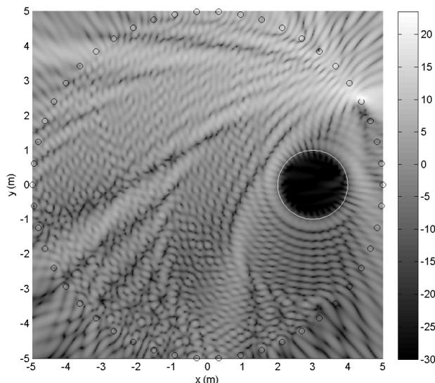
**Figure 5: Reproduction error in dB at 1 kHz,  $R_S = 5.1$  m,  $R_Z=1$ m. LWE = 1.3**
