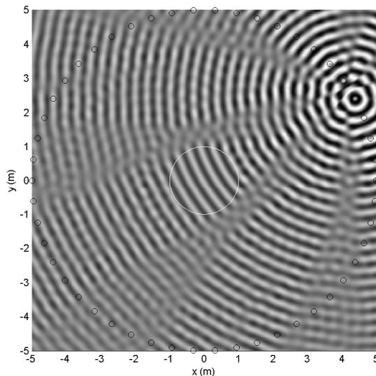
**Figure 3: Sound field at 1 kHz,  $R_S = 5.1$  m  $R_Z=1$ m at origin**
