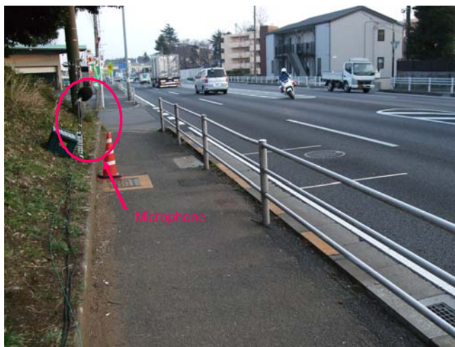
Figure 1.1 – View of road traffic noise being measured
