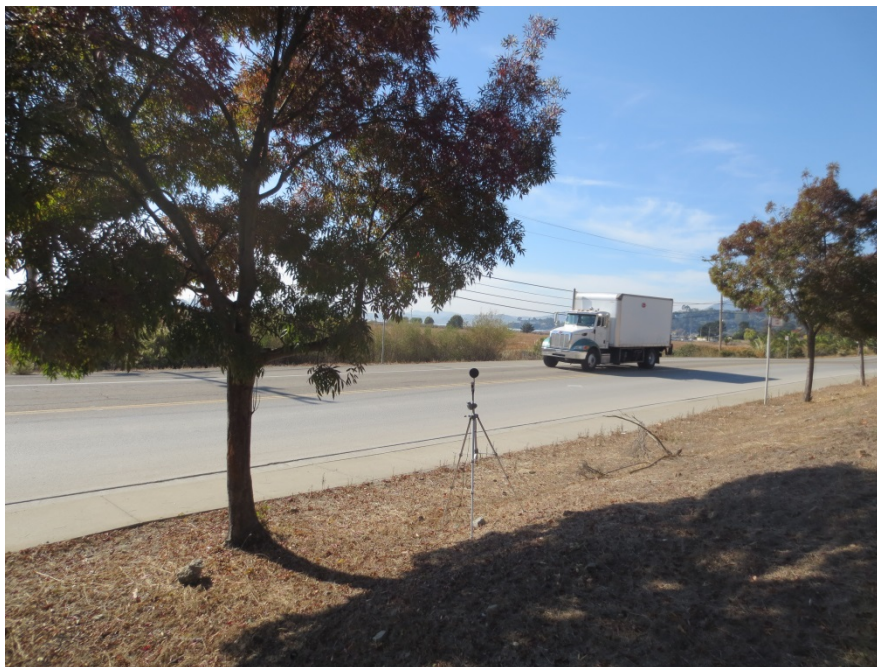
Figure 3 - Pass-by microphone located a site along Point San Pedro Road 7.5 m from the center of the near, westbound lane of travel
