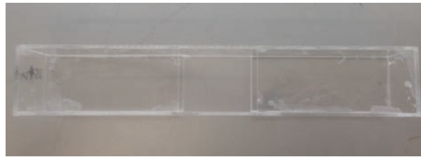
Figure 2 – A resonance tube (inside: 40 mm × 40 mm × 250 mm, outside: 44 mm × 44 mm × 254 mm). It has a 40 mm × 50 mm hole at the middle of the side.
