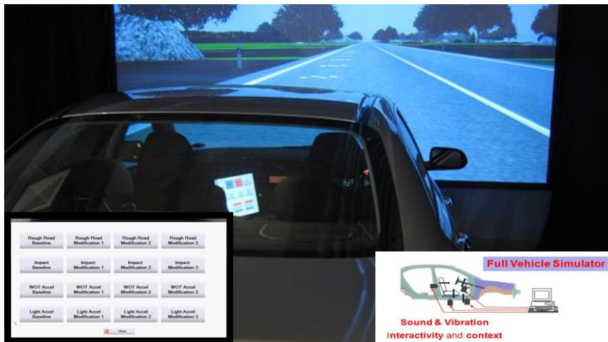
Figure 10 - Full Vehicle Simulator Cockpit & Visuals with touchscreen (left inset) & shaker schematic (right inset)
