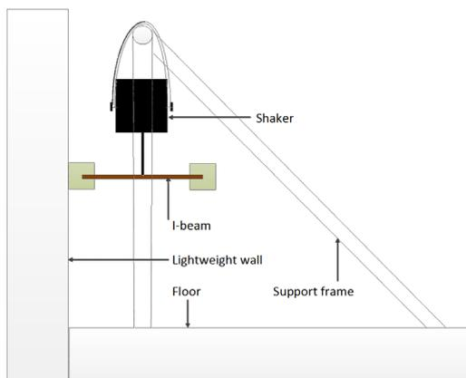
Figure 1 - Excitation concept with a shaker, beam with (on figure not visible) screws
