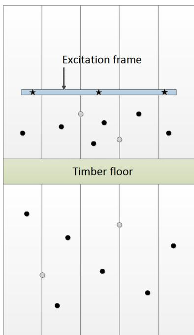
Figure 2 - Front view of the frame construction of upper and lower wall with excitation and principal measurement positions
