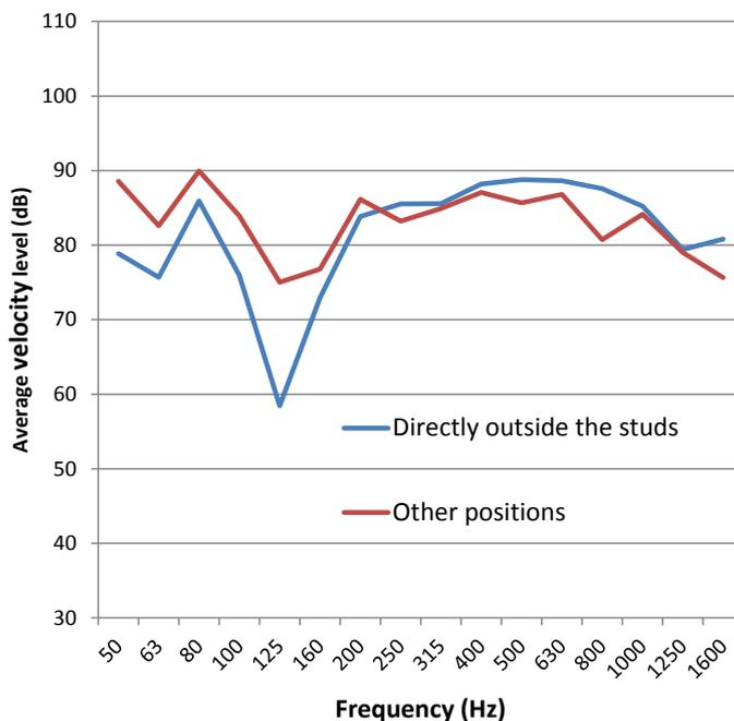
Figure 5 - Average velocity levels on the source area depending on accelerometer position relative to the framework, see figure 2
