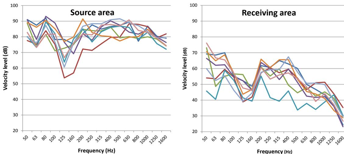
Figure 4a and b - Velocity levels, respectively on the source and receiving side of the T-junction
