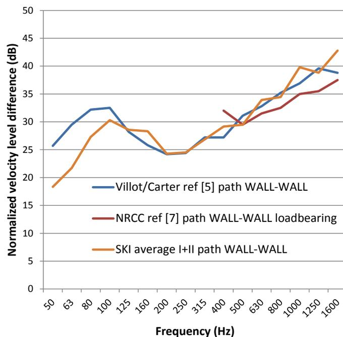
Figure 8 - Measured, normalized velocity level differences of timber-frame T-junctions with structural excitation
