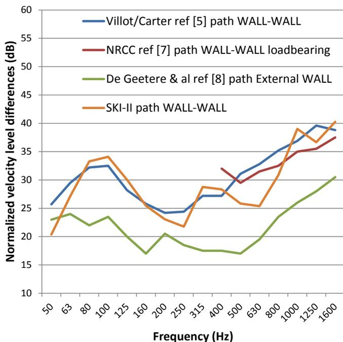
Figure 7 - Measured, normalized velocity level differences of timber-frame T-junctions
