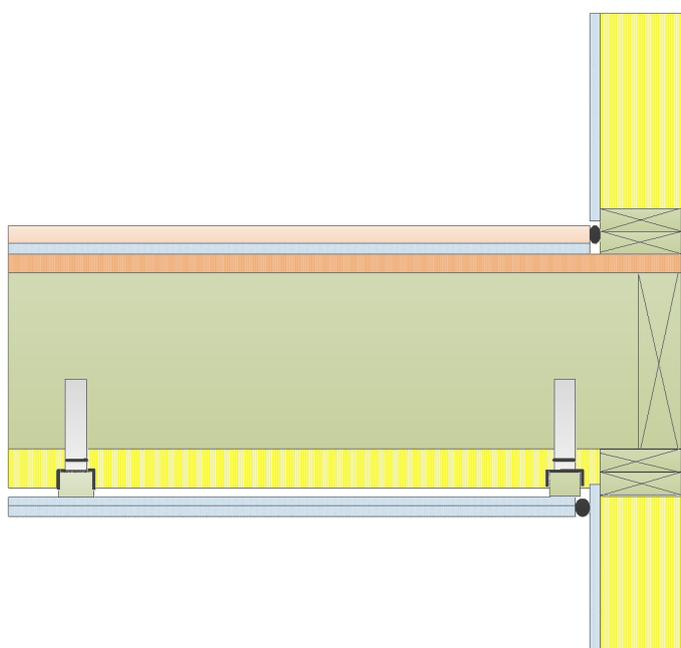
Figure 3 - T-junction between upper wall, floor construction and lower wall of measurement object "SKI"
