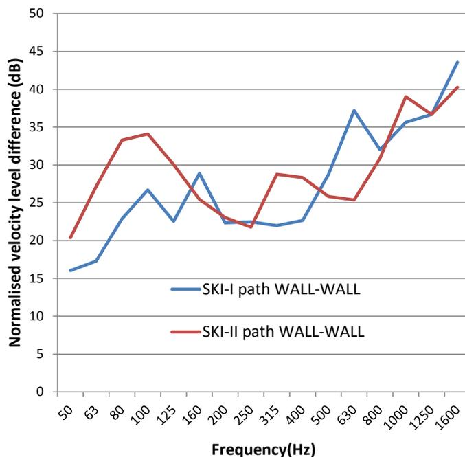
Figure 6 - Measured normalized velocity level differences of the two "SKI" T-junctions
