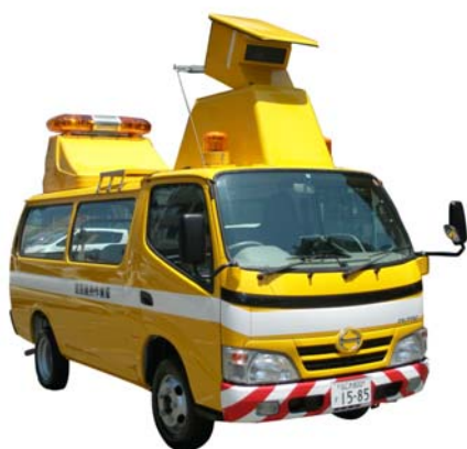
Figure 10 – Measuring car for roughness of road surface
