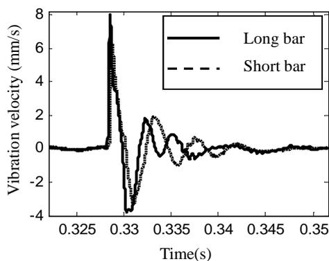
Figure 5 Longitudinal vibration velocity at the free ends of bars with different lengths
