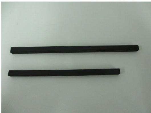
Figure 4 Viscoelastic long and short stick
