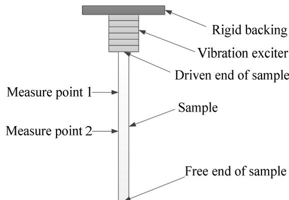
Figure 1 Wave-speed measurements diagram
