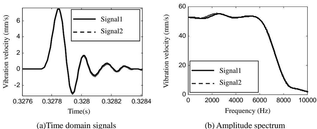
Figure 3 Butterworth broadband short pulse generated by vibration exciter
