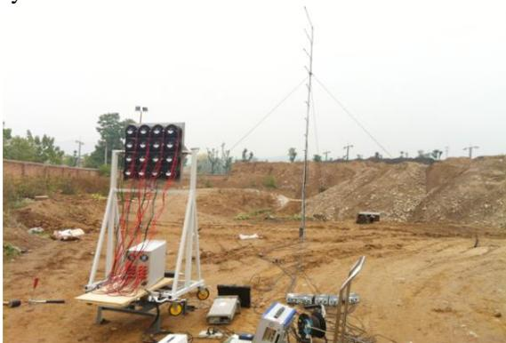
Figure 6-Experiment image of acoustic emission array
