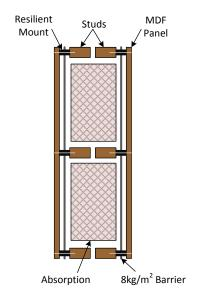
Figure 7 - Proposed separating wall design.
