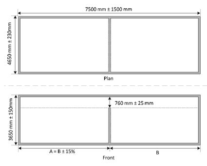
Figure 1 - Dimensions of test facility required by ASTM E1414
