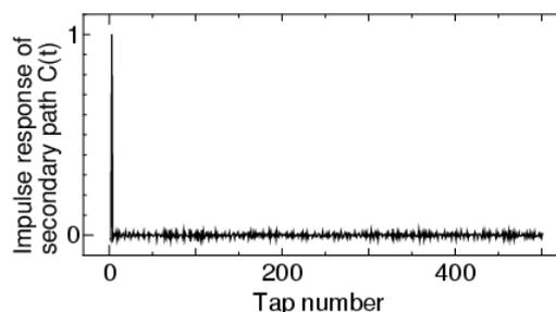
Figure 6 –Impulse response of the secondary path  $C(t)$  of the active noise control.
