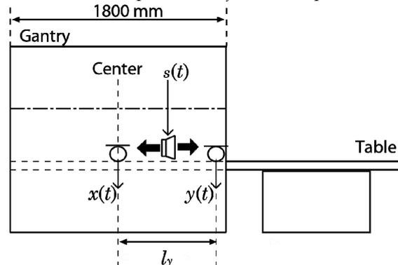
Figure 1 –The method for estimating the location of the apparent sound source.
