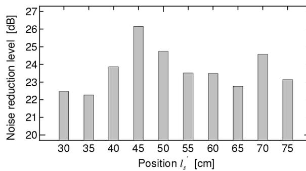
Figure 7 –Reduction level of the active noise control system for each position of the reference microphone.
