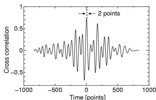
Figure 3 – Cross correlation function of the additively averaged waveforms  $x_0(t)$  and  $y_0(t)$ .
