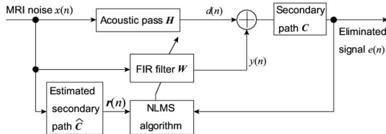
Figure 4 –Block diagram of the feedforward ANC system.
