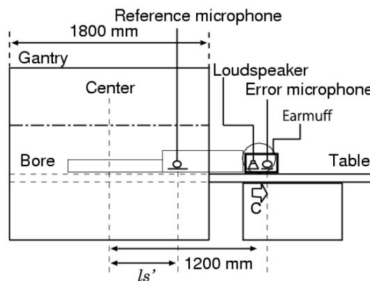
Figure 5 –The positional relation between the MRI equipment and the active noise control system in the case of a knee examination.
