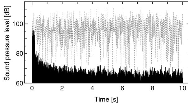
Figure 8 –Actual level of MRI acoustical noise (dashed line), and the reduced noise (solid line) ( $l_s' = 45$  cm).
