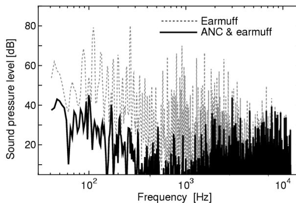
Figure 9 –Frequency characteristics of controlled noise ( $l_s' = 45$  cm).
