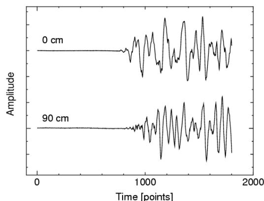
Figure 2 –Enlargement of the leading edges of the waveforms  $x_0(t)$  and  $y_0(t)$  of a burst wave.
