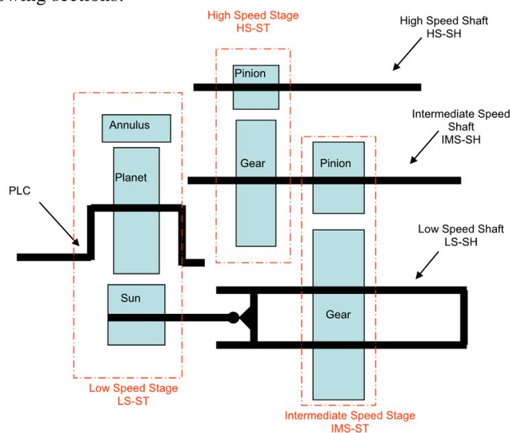
Figure 2 – Multi-stage gearbox arrangement (13)
