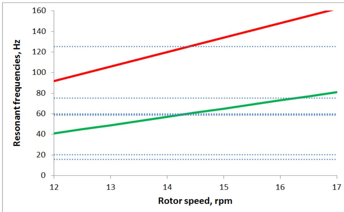
**Figure 5 – Example Campbell diagram which indicates GMF of the LSS and ISS (shown in green and red) in comparison with the dominant resonant frequencies (blue dotted lines). Intersections within the turbine operating rotor speed range indicate important radiating elements.**
