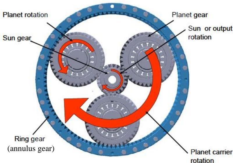
Figure 3 – Planetary stage of the gearbox and rotational directions (4)
