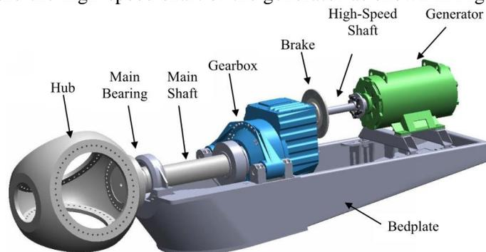
Figure 1 – Drivetrain configuration of a wind turbine (4)
