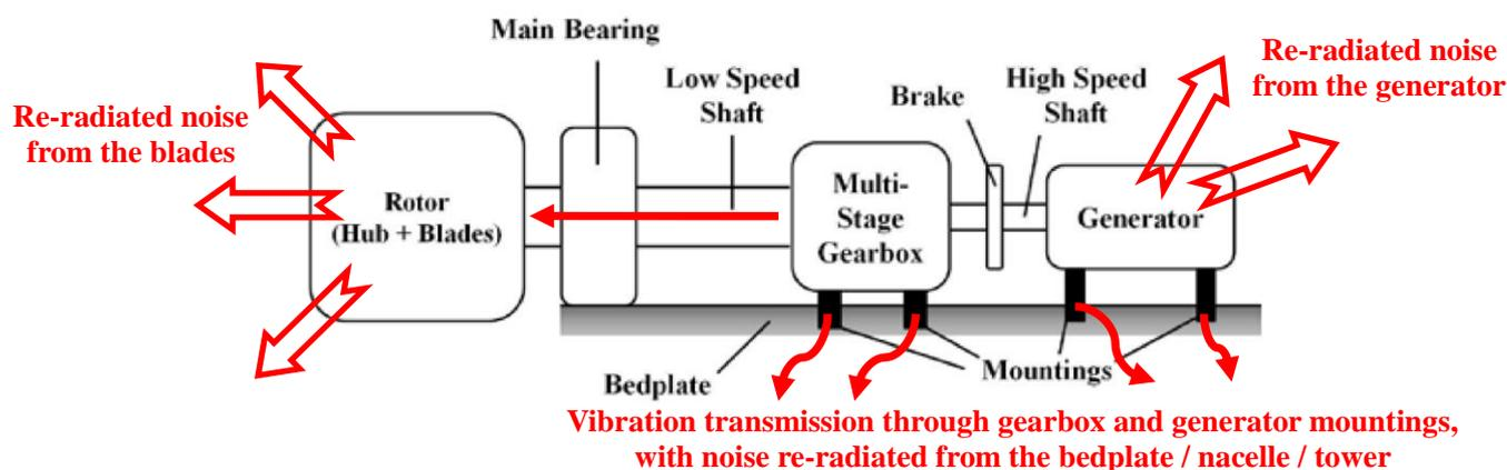
**Figure 6 – Drivetrain configuration of a wind turbine (5)**
