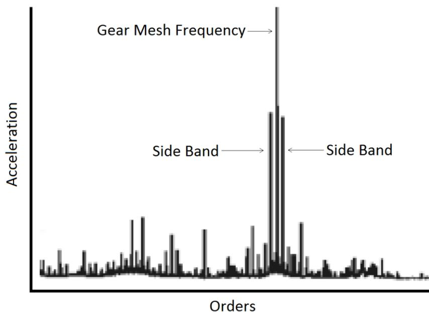
**Figure 4 – Order analysis (zoomed) showing the gear mesh frequency and side bands**
