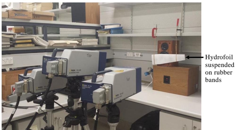
Figure 2 – The hydrofoil supported by rubber bands is indicated and the loudspeaker is directly behind the hydrofoil. The three laser vibrometer heads are in the foreground.
