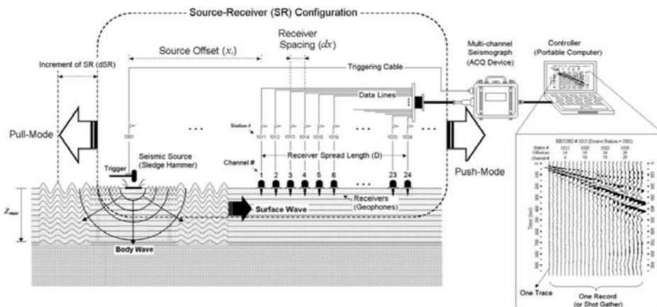
Figure 2 Typical MASW test setup
