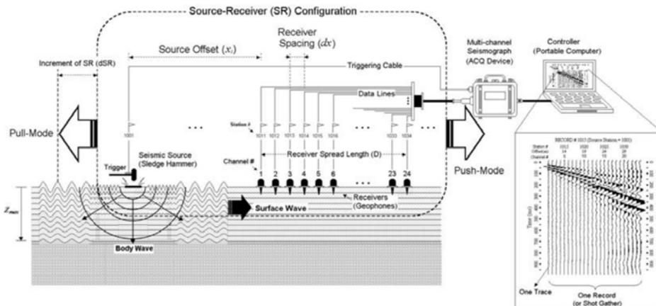
Figure 2 Typical MASW test setup
