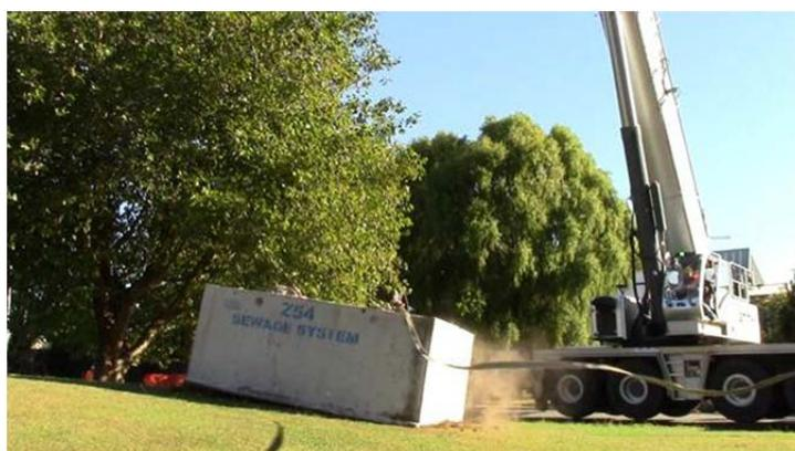
Figure 5 Impact testing using 16 tonne weight and an array of tri-axial accelerometers
