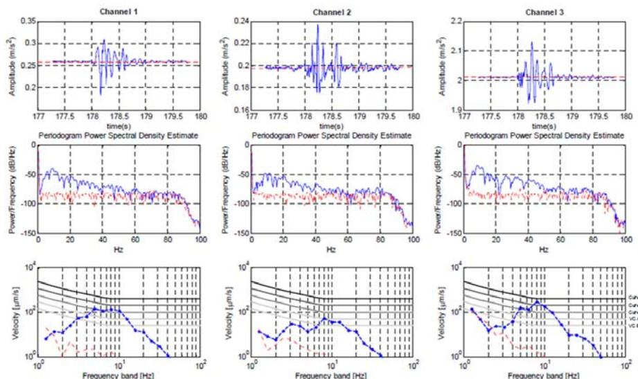
Figure 6 Typical measured ground-vibration response (Blue) vs background level (Red)
