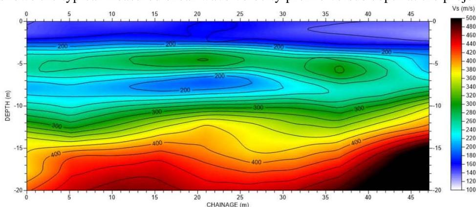
Figure 3 Section of shear wave velocity profile with depth
