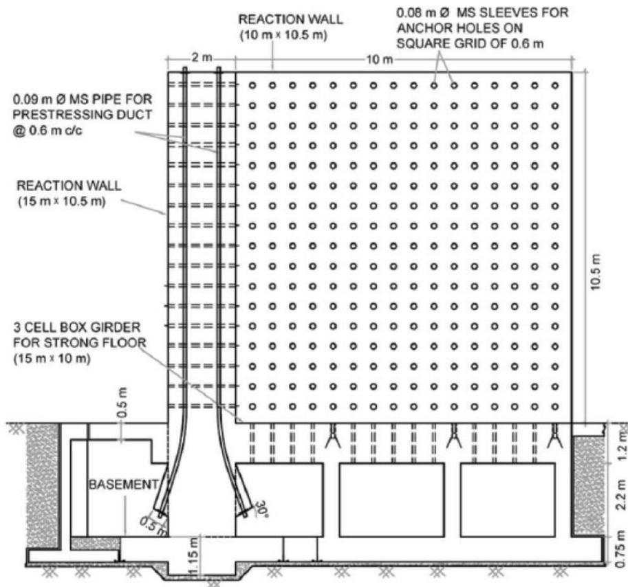
Figure 7 Typical section through the strong wall/floor
