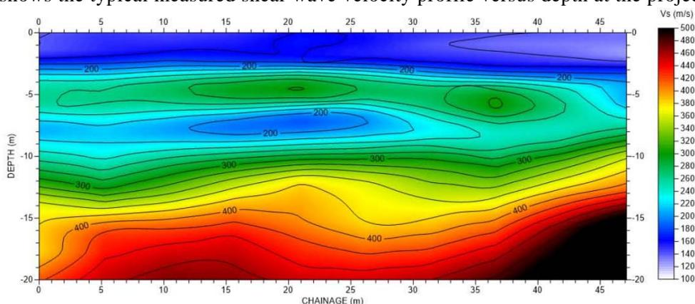
Figure 3 Section of shear wave velocity profile with depth
