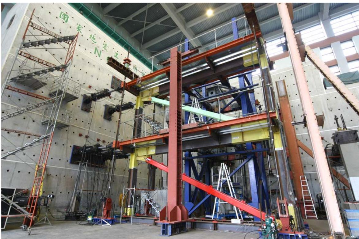
Figure 1 Quasi-static Testing (ncree.org.tw)
