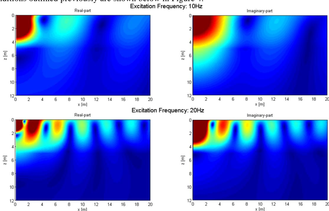
Figure 4 Real/Imaginary components of displacement due to a unit load at (0,0) cycling at 10Hz and 20Hz.
